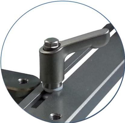
Adjust release levers to loosen slide bar
